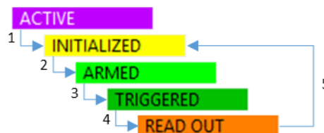
Figure 4-4. Acquisition Sequence in the TestMan Module
