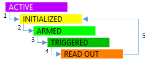
Figure 2-16. Instrument states during a standard acquisition sequence
