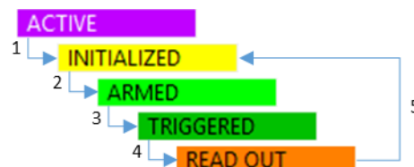
Figure 4-4. Acquisition Sequence in the TestMan Module
