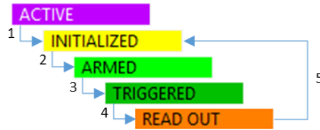
Figure 2-16. Instrument states during a standard acquisition sequence
