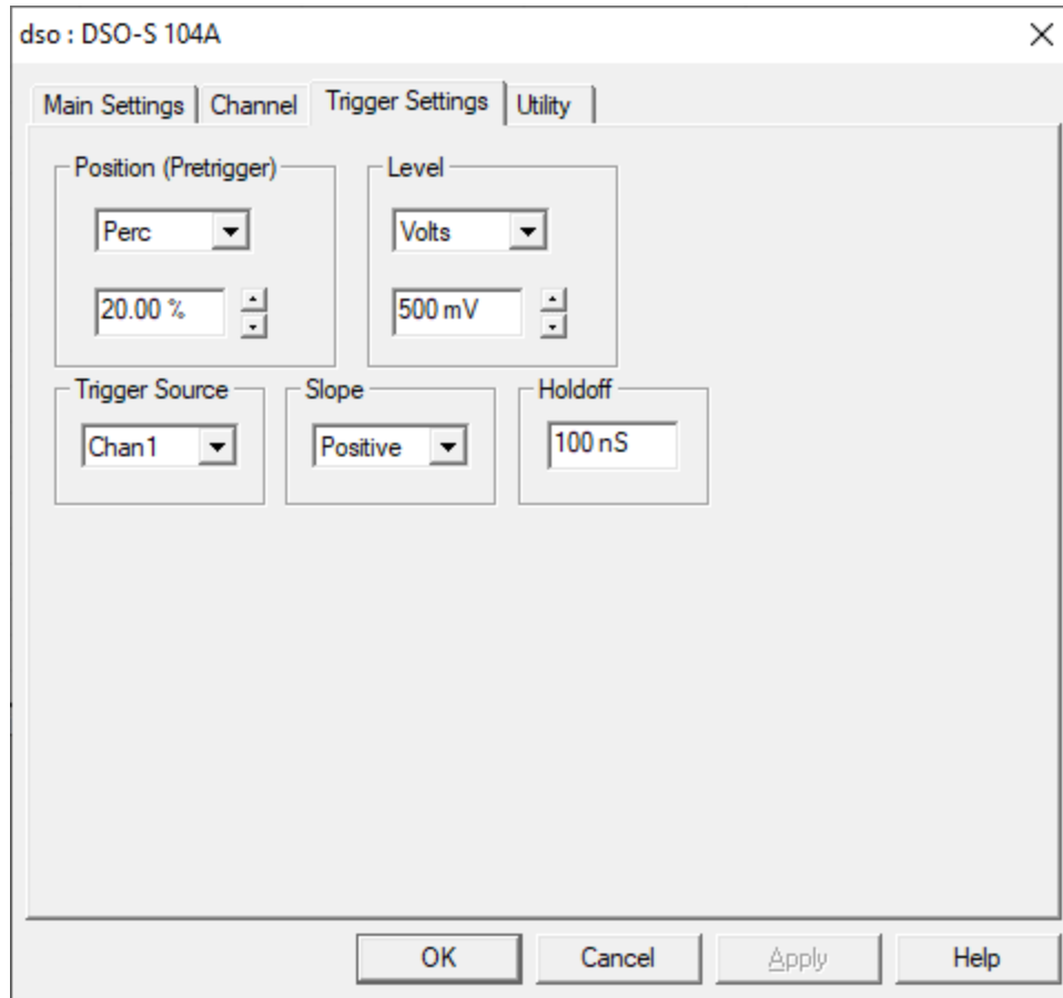
Figure 2-10. Oscilloscope trigger settings
