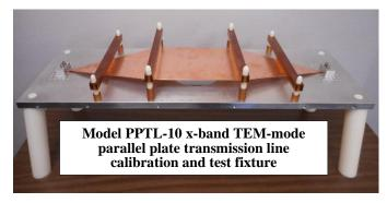
plate that can accommodate structures with diameters up to 6 inches. It is also offered in a version that accommodates free-field sensors with center ground planes and mounting shafts up to ¼ inch diameter.
